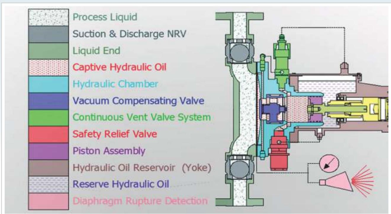
The diaphragm is hydraulically actuated. Its function is basically that of a partition. Hence, very high pumping pressures can be attained.
