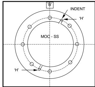
tighten clamping bolts **evenly**. [In case of diaphragm pumps with plastic heads bolts should not be over-tightened to distort the plastic head.] **NOTE**
